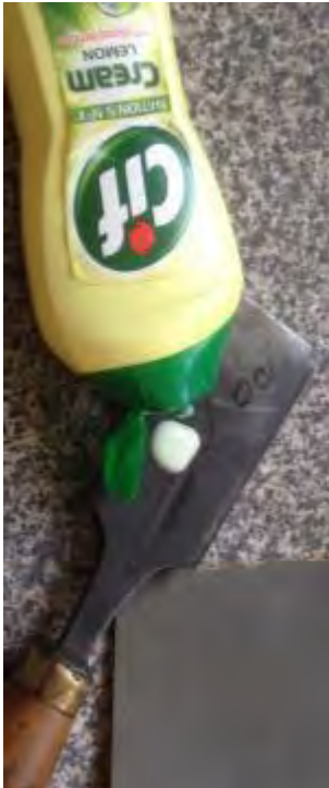
Sanded under running water with fine wet and dry sandpaper and Jif
