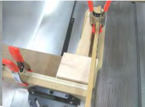
To safely cut these angles at the table saw, I temporarily secure a cradle to the mitre gauge to support the piece through out the cuts. Note that I'm using the same wooden strip clamped to the saw blade to align this latter with the cut line to set the angle of the mitre gauge.
