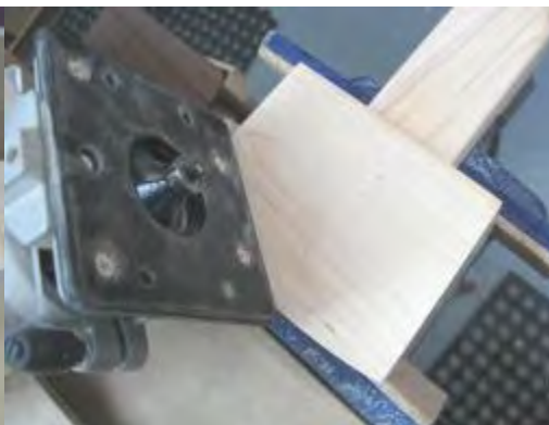
The head swung in the bench vise, I'm getting ready to chamfer the three upper edges of each cheek with my trim router outfitted with a chamfering bit, but in two passes because I want to minimize burn marks.
