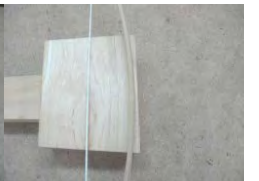
Here I'm tracing a line with my shop made curve drawing stick to complete the head. I don't mess with ugly tools!
