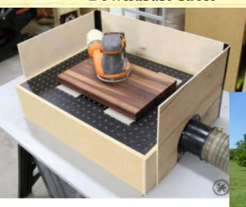
Sanding often leads to dust- unhealthy and a nuisance. This clever piece of kit sucks the dust downwards – not up as most such devices. Full details at DIY Downdraft Table for Sanding | How to Build Bingwides
