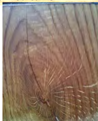
Medullary rays in oak – across the grain (above) and with the grain (below)
