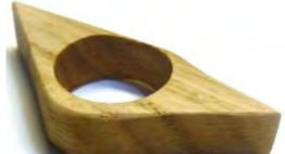
Use a discarded kitchen worktop insert (from where the sink goes) to make one or more chopping boards. A jig saw needed for the cut out, simple gouging to smooth the edges
