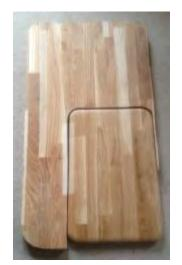
Cut out the piece worktop with a jigsaw and round the edges with simple gouge work. Smooth the whole with sandpaper
