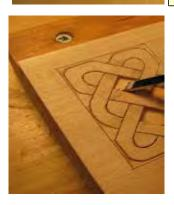
Bevel 3. down, remove the background areas that surround the shape. Use both chisels and gouges for this and try to maintain consistent depth of cut. Don't fret too much if it's not perfect; you'll have another shot at it as you're finishing the carving.
