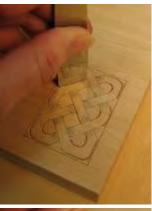
1. Lay out the design on your workpiece and define the outer and inner edges of the shape with chisels and gouges. Shade the under parts of the knots with pencil to help avoid accidentally cutting across the "over" parts.
