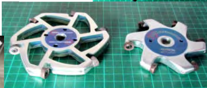
The replaceable carbide heads
