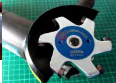
The replaceable carbide heads
